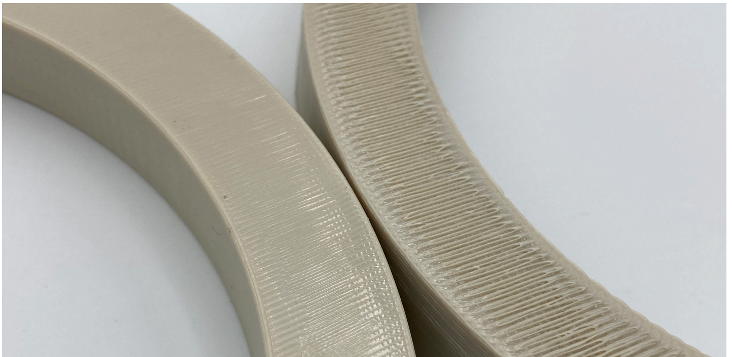
Left: 0.4mm nozzle Right: 0.6mm nozzle
